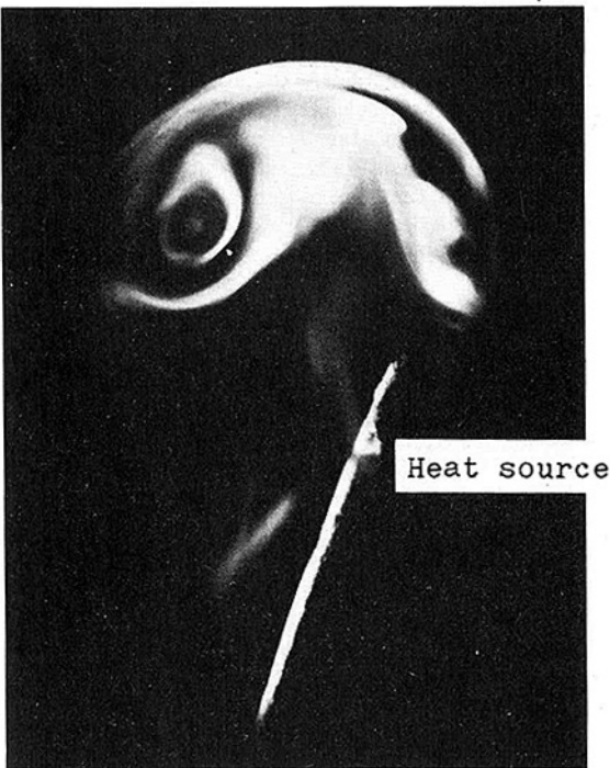
Fig. 2 (b) Vortex rising above the source, flow angle 20 deg, air velocity 22.4 cm/s
