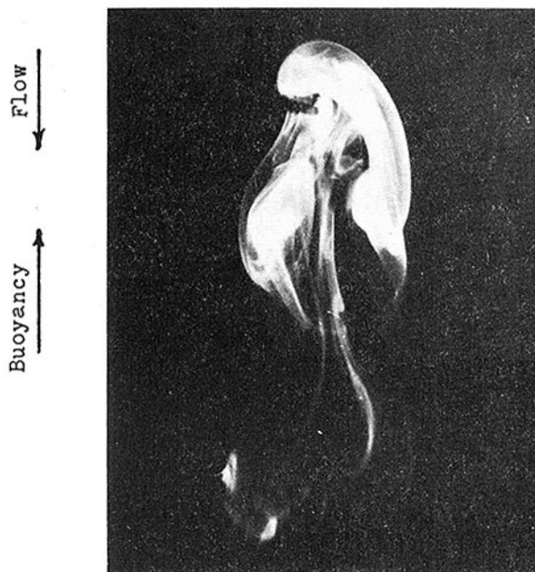
Fig. 1 (b) Spiral vortex shedding, air velocity 25.5 cm/s
